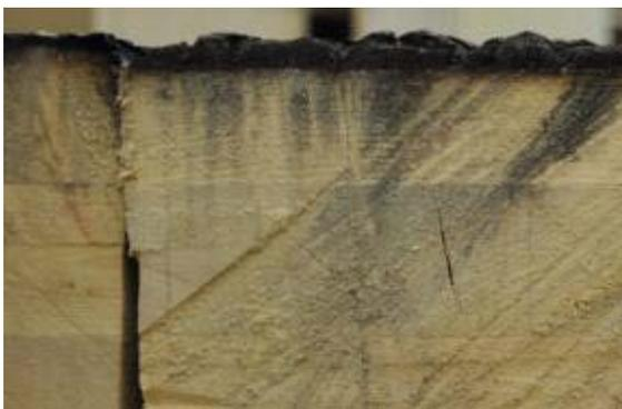
Figure 7: Burning pattern typical CLT panels.
