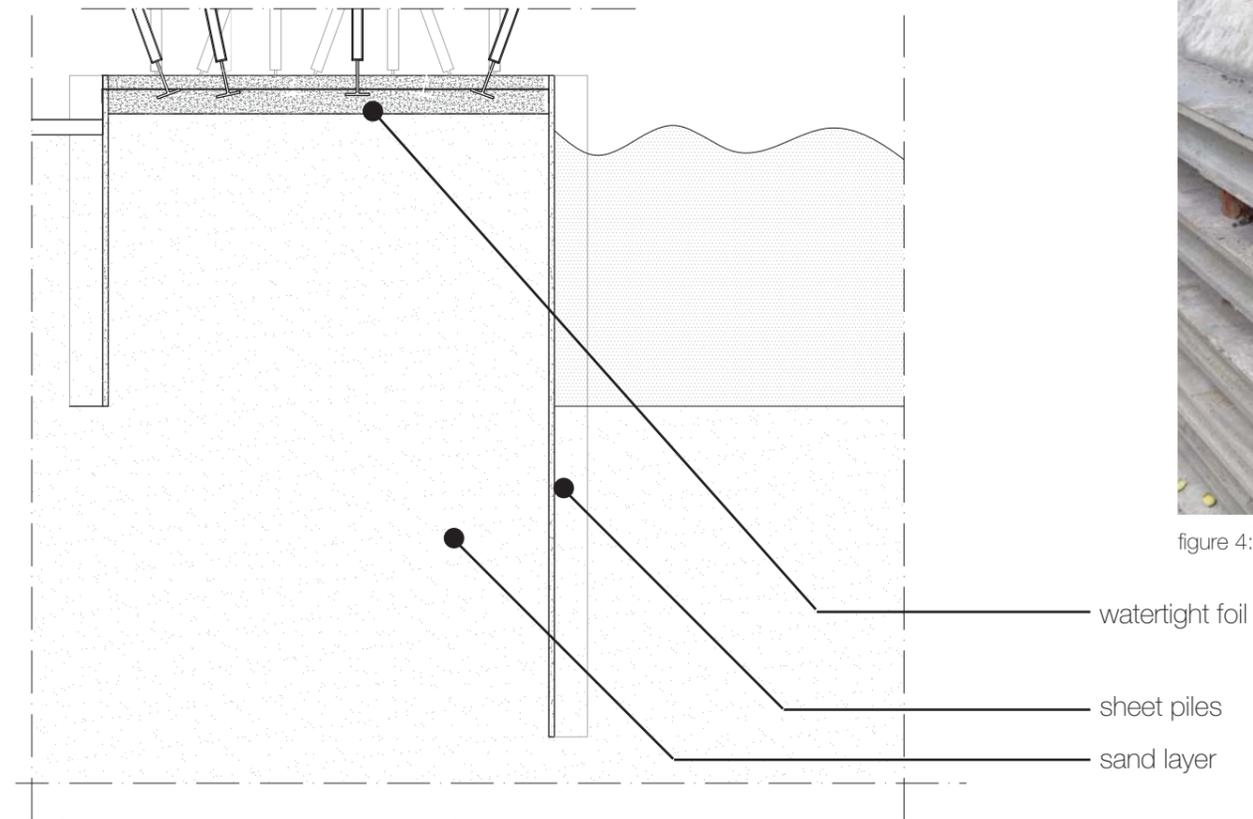
figure 3: schematic section of the building foundation. scale 1:50
